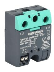
Gefran solid state relay, panel mount, 20-260 VAC input voltage, SPST, (1) N.O. SCR, 90A contact rating, 48-600 VAC load voltage, push-in spring, overvoltage protection. Thermal mounting pad included.
