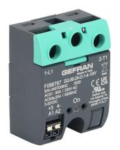
Gefran solid state relay, panel mount, 3-32 VDC input voltage, SPST, (1) N.O. SCR, 90A contact rating, 24-230 VAC load voltage, push-in spring, overvoltage protection. Thermal mounting pad included.
