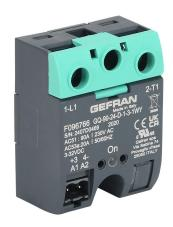
Gefran solid state relay, panel mount, 3-32 VDC input voltage, SPST, (1) N.O. SCR, 90A contact rating, 24-230 VAC load voltage, screw terminal(s), overvoltage protection. Thermal mounting pad included.
