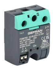
Gefran solid state relay, panel mount, 20-260 VAC input voltage, SPST, (1) N.O. SCR, 90A contact rating, 24-230 VAC load voltage, push-in spring, overvoltage protection. Thermal mounting pad included.
