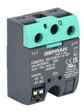
Gefran solid state relay, panel mount, 3-32 VDC input voltage, SPST, (1) N.O. SCR, 75A contact rating, 48-600 VAC load voltage, push-in spring, overvoltage protection. Thermal mounting pad included.
