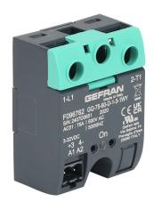
Gefran solid state relay, panel mount, 3-32 VDC input voltage, SPST, (1) N.O. SCR, 75A contact rating, 48-600 VAC load voltage, screw terminal(s), overvoltage protection. Thermal mounting pad included.
