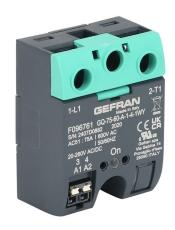
Gefran solid state relay, panel mount, 20-260 VAC input voltage, SPST, (1) N.O. SCR, 75A contact rating, 48-600 VAC load voltage, push-in spring, overvoltage protection. Thermal mounting pad included.
