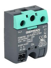
Gefran solid state relay, panel mount, 20-260 VAC input voltage, SPST, (1) N.O. SCR, 75A contact rating, 48-600 VAC load voltage, screw terminal(s), overvoltage protection. Thermal mounting pad included.
