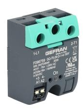
Gefran solid state relay, panel mount, 3-32 VDC input voltage, SPST, (1) N.O. SCR, 75A contact rating, 24-230 VAC load voltage, push-in spring, overvoltage protection. Thermal mounting pad included.
