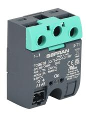
Gefran solid state relay, panel mount, 3-32 VDC input voltage, SPST, (1) N.O. SCR, 75A contact rating, 24-230 VAC load voltage, screw terminal(s), overvoltage protection. Thermal mounting pad included.
