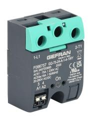
Gefran solid state relay, panel mount, 20-260 VAC input voltage, SPST, (1) N.O. SCR, 75A contact rating, 24-230 VAC load voltage, push-in spring, overvoltage protection. Thermal mounting pad included.
