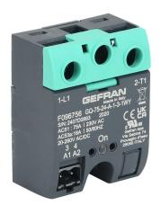
Gefran solid state relay, panel mount, 20-260 VAC input voltage, SPST, (1) N.O. SCR, 75A contact rating, 24-230 VAC load voltage, screw terminal(s), overvoltage protection. Thermal mounting pad included.
