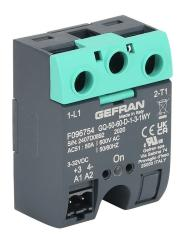
Gefran solid state relay, panel mount, 3-32 VDC input voltage, SPST, (1) N.O. SCR, 50A contact rating, 48-600 VAC load voltage, screw terminal(s), overvoltage protection. Thermal mounting pad included.
