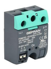
Gefran solid state relay, panel mount, 20-260 VAC input voltage, SPST, (1) N.O. SCR, 50A contact rating, 48-600 VAC load voltage, push-in spring, overvoltage protection. Thermal mounting pad included.
