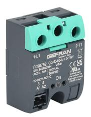
Gefran solid state relay, panel mount, 20-260 VAC input voltage, SPST, (1) N.O. SCR, 50A contact rating, 48-600 VAC load voltage, screw terminal(s), overvoltage protection. Thermal mounting pad included.
