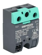
Gefran solid state relay, panel mount, 3-32 VDC input voltage, SPST, (1) N.O. SCR, 50A contact rating, 24-230 VAC load voltage, screw terminal(s), overvoltage protection. Thermal mounting pad included.
