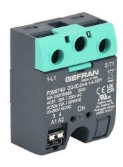
Gefran solid state relay, panel mount, 20-260 VAC input voltage, SPST, (1) N.O. SCR, 50A contact rating, 24-230 VAC load voltage, push-in spring, overvoltage protection. Thermal mounting pad included.
