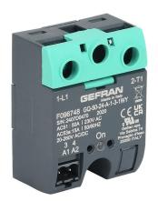
Gefran solid state relay, panel mount, 20-260 VAC input voltage, SPST, (1) N.O. SCR, 50A contact rating, 24-230 VAC load voltage, screw terminal(s), overvoltage protection. Thermal mounting pad included.
