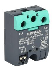
Gefran solid state relay, panel mount, 3-32 VDC input voltage, SPST, (1) N.O. SCR, 25A contact rating, 48-600 VAC load voltage, push-in spring, overvoltage protection. Thermal mounting pad included.
