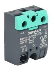
Gefran solid state relay, panel mount, 3-32 VDC input voltage, SPST, (1) N.O. SCR, 25A contact rating, 48-600 VAC load voltage, screw terminal(s), overvoltage protection. Thermal mounting pad included.
