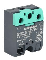
Gefran solid state relay, panel mount, 20-260 VAC input voltage, SPST, (1) N.O. SCR, 25A contact rating, 48-600 VAC load voltage, screw terminal(s), overvoltage protection. Thermal mounting pad included.
