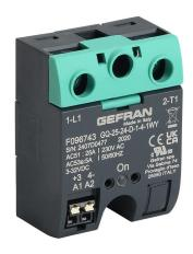
Gefran solid state relay, panel mount, 3-32 VDC input voltage, SPST, (1) N.O. SCR, 25A contact rating, 24-230 VAC load voltage, push-in spring, overvoltage protection. Thermal mounting pad included.
