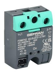
Gefran solid state relay, panel mount, 3-32 VDC input voltage, SPST, (1) N.O. SCR, 25A contact rating, 24-230 VAC load voltage, screw terminal(s), overvoltage protection. Thermal mounting pad included.
