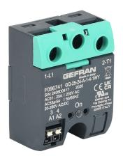
Gefran solid state relay, panel mount, 20-260 VAC input voltage, SPST, (1) N.O. SCR, 25A contact rating, 24-230 VAC load voltage, push-in spring, overvoltage protection. Thermal mounting pad included.
