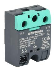
Gefran solid state relay, panel mount, 20-260 VAC input voltage, SPST, (1) N.O. SCR, 25A contact rating, 24-230 VAC load voltage, screw terminal(s), overvoltage protection. Thermal mounting pad included.
