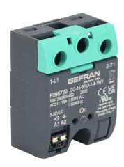
Gefran solid state relay, panel mount, 3-32 VDC input voltage, SPST, (1) N.O. SCR, 15A contact rating, 48-600 VAC load voltage, push-in spring, overvoltage protection. Thermal mounting pad included.
