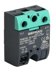
Gefran solid state relay, panel mount, 3-32 VDC input voltage, SPST, (1) N.O. SCR, 15A contact rating, 48-600 VAC load voltage, screw terminal(s), overvoltage protection. Thermal mounting pad included.
