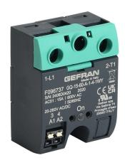
Gefran solid state relay, panel mount, 20-260 VAC input voltage, SPST, (1) N.O. SCR, 15A contact rating, 48-600 VAC load voltage, push-in spring, overvoltage protection. Thermal mounting pad included.
