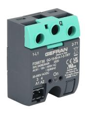
Gefran solid state relay, panel mount, 20-260 VAC input voltage, SPST, (1) N.O. SCR, 15A contact rating, 48-600 VAC load voltage, screw terminal(s), overvoltage protection. Thermal mounting pad included.
