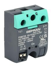
Gefran solid state relay, panel mount, 3-32 VDC input voltage, SPST, (1) N.O. SCR, 15A contact rating, 24-230 VAC load voltage, push-in spring, overvoltage protection. Thermal mounting pad included.
