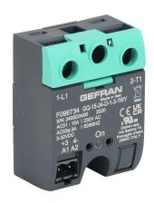
Gefran solid state relay, panel mount, 3-32 VDC input voltage, SPST, (1) N.O. SCR, 15A contact rating, 24-230 VAC load voltage, screw terminal(s), overvoltage protection. Thermal mounting pad included.
