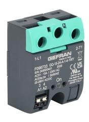
Gefran solid state relay, panel mount, 20-260 VAC input voltage, SPST, (1) N.O. SCR, 15A contact rating, 24-230 VAC load voltage, push-in spring, overvoltage protection. Thermal mounting pad included.
