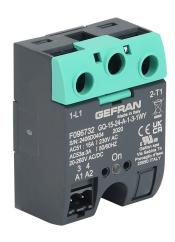
Gefran solid state relay, panel mount, 20-260 VAC input voltage, SPST, (1) N.O. SCR, 15A contact rating, 24-230 VAC load voltage, screw terminal(s), overvoltage protection. Thermal mounting pad included.
