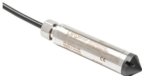
ProSense hydrostatic submersible level transmitter, 0 to 50 psig (115.5ft of water column) sensing range, 4-20 mA, 0.825in diameter housing, shielded and vented 140ft cable, hazardous location rated.
