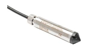
ProSense hydrostatic submersible level transmitter, 0 to 50 psig (115.5ft of water column) sensing range, 4-20 mA, 0.825in diameter housing, shielded and vented 140ft cable, hazardous location rated.
