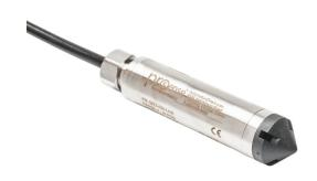
ProSense hydrostatic submersible level transmitter, 0 to 30 psig (69.2ft of water column) sensing range, 4-20 mA, 0.825in diameter housing, shielded and vented 100ft cable, hazardous location rated.
