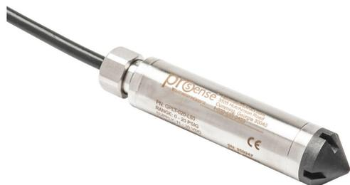
ProSense hydrostatic submersible level transmitter, 0 to 20 psig (46.1ft of water column) sensing range, 4-20 mA, 0.825in diameter housing, shielded and vented 60ft cable, hazardous location rated.
