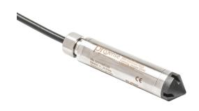
ProSense hydrostatic submersible level transmitter, 0 to 20 psig (46.1ft of water column) sensing range, 4-20 mA, 0.825in diameter housing, shielded and vented 60ft cable, hazardous location rated.
