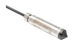
ProSense hydrostatic submersible level transmitter, 0 to 15 psig (34.6ft of water column) sensing range, 4-20 mA, 0.825in diameter housing, shielded and vented 60ft cable, hazardous location rated.
