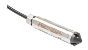
ProSense hydrostatic submersible level transmitter, 0 to 5 psig (11.5ft of water column) sensing range, 4-20 mA, 0.825in diameter housing, shielded and vented 30ft cable, hazardous location rated.
