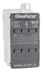
Gladiator enclosed terminal block, finger-safe, 510A, 1-pole, line side: 2 openings accept 250 kcmil to 4 AWG, load side: 2 openings accept 250 kcmil to 4 AWG, DIN rail or panel mount, UL 1059 recognized.
