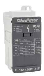
Gladiator enclosed terminal block, finger-safe, 420A, 1-pole, line side: 1 opening accepts flat busbar, load side: 2 openings accept 2 AWG to 14 AWG & 5 openings accept 6 AWG to 14 AWG & 4 openings accept 8 AWG to 14 AWG, DIN rail or panel mount, UL 1059 recognized.
