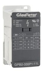
Gladiator enclosed terminal block, finger-safe, 335A, 1-pole, line side: 1 opening accepts 400 kcmil to 3/0 AWG, load side: 2 openings accept 2 AWG to 14 AWG & 5 openings accept 6 AWG to 14 AWG & 4 openings accept 8 AWG to 14 AWG, DIN rail or panel mount.
