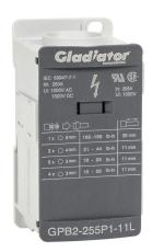
Gladiator enclosed terminal block, finger-safe, 225A, 1-pole, line side: 1 opening accepts 250 kcmil to 2 AWG, load side: 2 openings accept 2 AWG to 14 AWG & 5 openings accept 6 AWG to 14 AWG & 4 openings accept 8 AWG to 14 AWG, DIN rail or panel mount.
