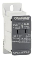
Gladiator enclosed terminal block, finger-safe, 250A, 1-pole, line side: 1 opening accepts flat busbar, load side: 6 openings accept 6 AWG to 14 AWG, DIN rail or panel mount, UL 1059 recognized.
