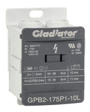
Gladiator enclosed terminal block, finger-safe, 175A, 1-pole, line side: 2 openings accept 2/0 AWG to 6 AWG, load side: 10 openings accept 6 AWG to 14 AWG, DIN rail or panel mount, UL 1059 recognized.
