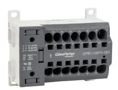
Gladiator enclosed terminal block, finger-safe, 130A, 1-pole, line side: 2 (screw) openings accept 1 AWG to 8 AWG & 2 openings accept 6 AWG to 16 AWG, load side: 12 openings accept 8 AWG to 16 AWG, DIN rail or panel mount, UL 1059 recognized.
