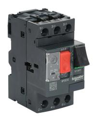
Schneider Electric Easy TeSys series manual motor protector, pushbutton, 25A, thermal overload, 20-25 adjustable, 327A instantaneous trip rating, 45mm frame.
