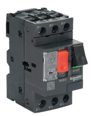
Schneider Electric Easy TeSys series manual motor protector, pushbutton, 23A, thermal overload, 17-23 adjustable, 327A instantaneous trip rating, 45mm frame.
