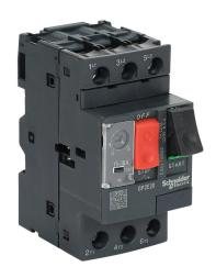
Schneider Electric Easy TeSys series manual motor protector, pushbutton, 18A, thermal overload, 13-18 adjustable, 223A instantaneous trip rating, 45mm frame.
