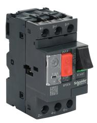
Schneider Electric Easy TeSys series manual motor protector, pushbutton, 14A, thermal overload, 9-14 adjustable, 170A instantaneous trip rating, 45mm frame.
