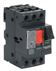
Schneider Electric Easy TeSys series manual motor protector, pushbutton, 10A, thermal overload, 6-10 adjustable, 138A instantaneous trip rating, 45mm frame.
